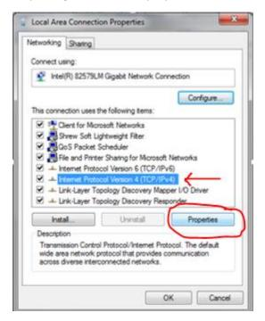
Step 4: Change your settings as needed. For most of Codi machine networks the subnet is 2 and device addresses that are already in use are .10, .20, .30, .40 etc... so using an IP of .99 is usually safe.
